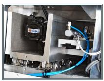
Figure 3. Rear view of the Versamill 4X-100 showing cast aluminum-alloy castings linear guide ways
