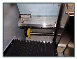
Figure 6. Internal view of the versamill 5X-200 showing use of precision ballscrews w/antibacklash nut, large way-surface with linear guide and protective coverings. All elements found in "large-format" high-speed industrial machines but less common in a DMC.
