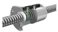
Figure 4. Figure 4. This cutaway drawing of a THK SBN ballscrew shows the main components of a typical ballscrew including the screw itself, a nut and the balls, which roll between the nut, screw and grooves.
