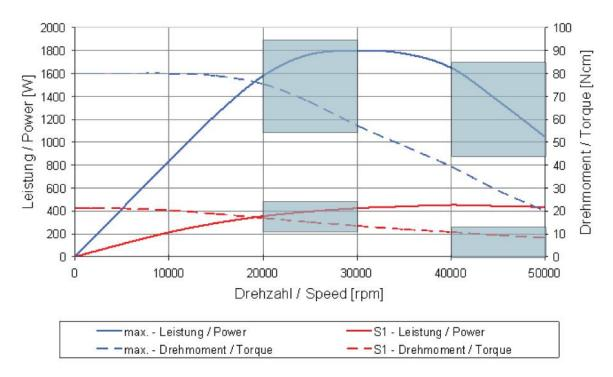
@ 45,000 rpm (the most useful speed range) - at MAXIMUM rating. Further The AC spindle torque drops to a mere 9Ncm just over 40,000 rpm S1 – continuous duty rating.
