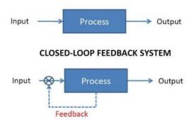
Most modern closed-loop CNC systems are able to provide very close resolution of 0.0001 of an inch. Closed-looped systems require more control devices and circuitry in order for them to implement both position and velocity control. This makes them more complex and more expensive than the open-loop system.
